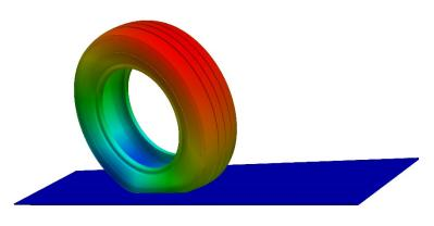
Fig. 1: Simulating contact of rolling tire and roadway surface.
