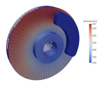
Fig. 2: Brake disc: contact with frictional heating.
